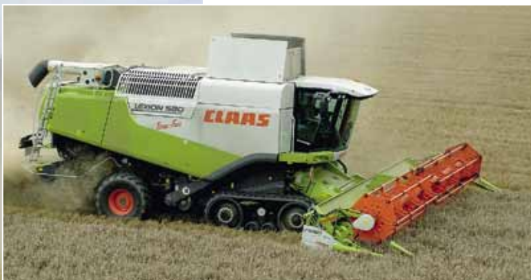
Despite other quite drastic equipment changes at Farmeco, the firm has always stuck with Claas combines. The latest is a Lexion 580 with 9m header and equipped with Terra-Tracs.
