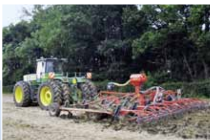
The original JD 9420 was replaced by a new, dualled-up JD 9520, which Mr Challen says was still the cheapest horsepower available at the time. The dual wheels, however, took the tractor to an overall width of 4m.
