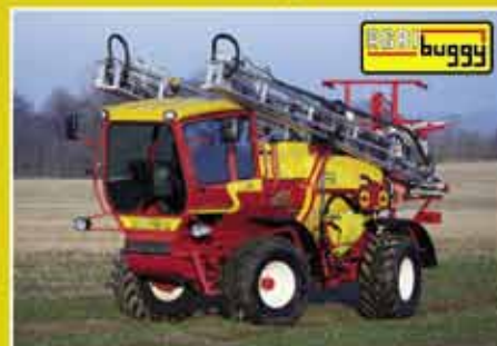
The most versatile of LGP self-propelled sprayers with 2500 litres and up to 32 metres
