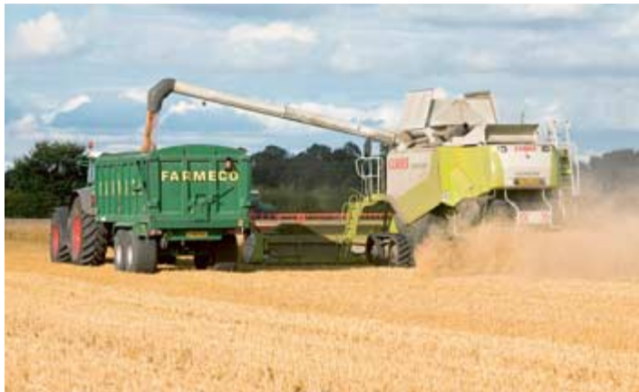
The combine's auger allows the grain cart tractor and trailer to run in the 8m wide CTF track, so the land in between is 'untrafficked'.
