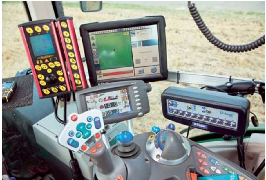
Fendt tractor cab mission control centre: Along with the tractor’s own Variotronic terminal, the cab hosts the drill controller, FmX screen and sprayer switch box. All of these items work together in the controlled-traffic system.
