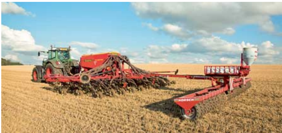
Direct drilling means all crops are established by one man and one tractor – Fendt 933, Väderstad Seed Hawk seed/fert drill and Simba Horsch Optipack. The 8m wide Seed Hawk drill sets the track width for the following fieldwork.
