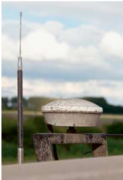
Trimble GPS antenna and radio aerial on the tractor roof receive signals from the on-farm RTK base station.
